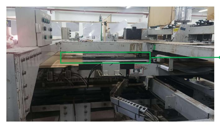
POSSIBLE PLACEMENT OF RUBBER ROLLER IN MACHINE GLUING 3 TO FLATTEN THE WARP ITEM
